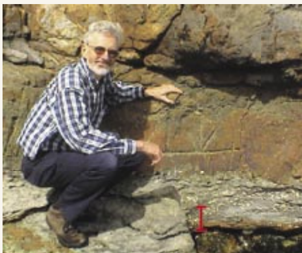
Figure 14: The sea level benchmark on the Isle of the Dead, Port Arthur, Tasmania, which was struck on 1 July 1841. Sea level measurements at that time and at the end of the 20th century have indicated a relative rise in mean sea level of 13.5 cm, as shown by the red bar superimposed below the benchmark (ACE CRC).
