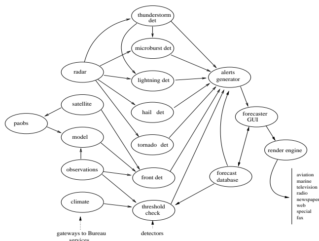
Figure 3: Example set of agents and their relationships in the desired network. The set of detector agents and gateway agents are indicated. Many other possible agent types and interactions are not shown for simplicity.
